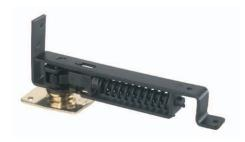
The Non-Hold Open pivot has the same performance criteria as our standard 7811/7812 series. It will carry a door size from 1 3/8" – 1 3/4" and 90lbs. Model# 7813 is with the Floor Plate; model# 7814 is with the Jamb Bracket.
