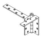
The hinge leaves are mortised in the door and jamb at the top corner, ANCHORING the door in the jamb. Provides increased reinforcement and support at the top corner where stress can occur due to high frequency service and abuse. Only available in Full Mortise type.
