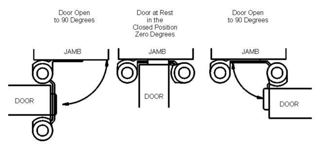
Permits doors to open in either direction and automatically return to closed position.
