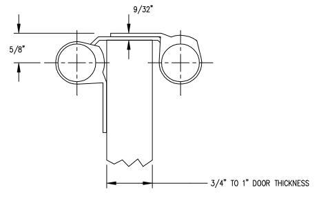
SCREWS: No. 7  $\times$  3/4" FLAT HEAD WOOD SCREWS
